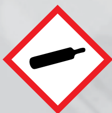
Gas under pressure
